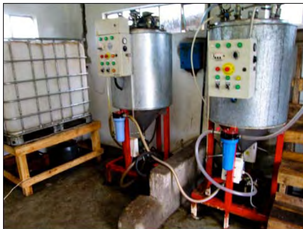
Left: A 400-liter batch biodiesel reactor near Naro Maru used by a local self help group and business to produce biodiesel from Croton and other oilseeds. Right: A local driver fills up with pure biodiesel (B100).
