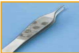
Stains on tweezers: Cause: Insufficient steam quality
