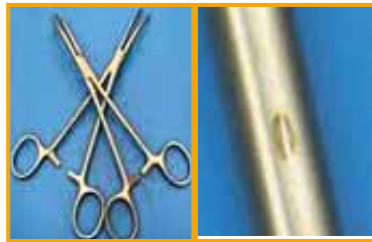
Contact corrosion: Stainless steel/Stainless steel
