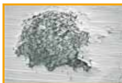
Pitting - seen under a scanning electron microscope - magnified 200 times
