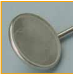
Stains on instruments. Cause: Dried water with high salt content
