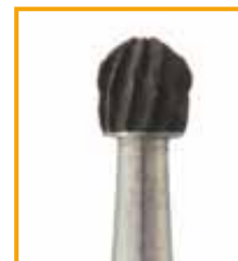
Corroded, worn out carbide drill head made of TC/CO. Cause: Application of an acid detergent.
