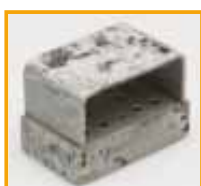
Severe material attack on the natural and color anodized aluminum surfaces of an instrument stand and containers. Cause: Overdosing of the otherwise material-compatible alkaline wash solution.
