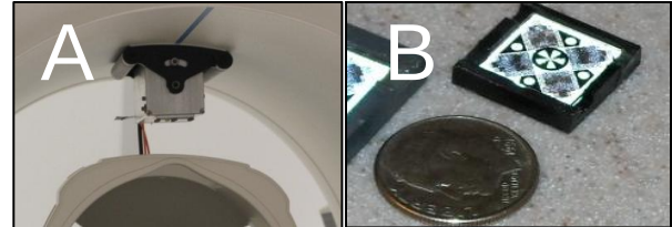
Fig. 1: Tracking system, consisting of A) the RGR camera in the scanner bore and B) the RGR target.
