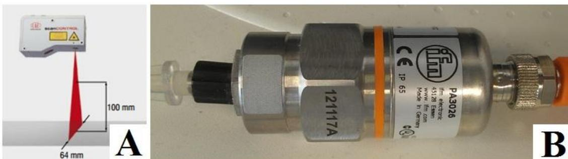
**Figure 54:** (A) A new laser sensor (LLT 2700-50(500), Micro Epsilon, Ortenburg, Germany) and (B) a new pressure sensor (PA3026, ifm electronic gmbh, Essen, Germany) of the new DIMPAST.
