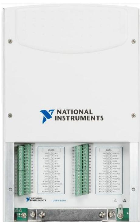
**Figure 19:** NI-USB 6251 Data-Acquisition Unit (National Instruments, NI-USB 6251 DAQ, Austin, USA).
