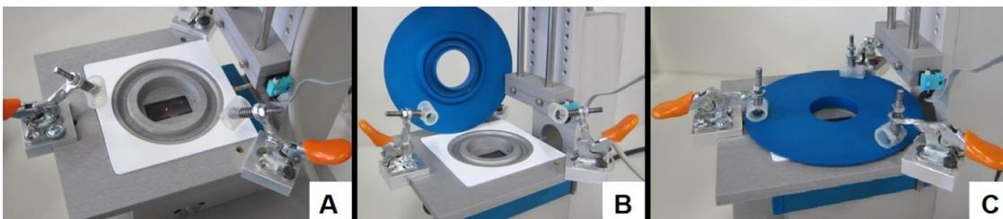
**Figure 18:** *Tissue Chamber (A) with fixing ring (B) fixed by clamps (C).*
