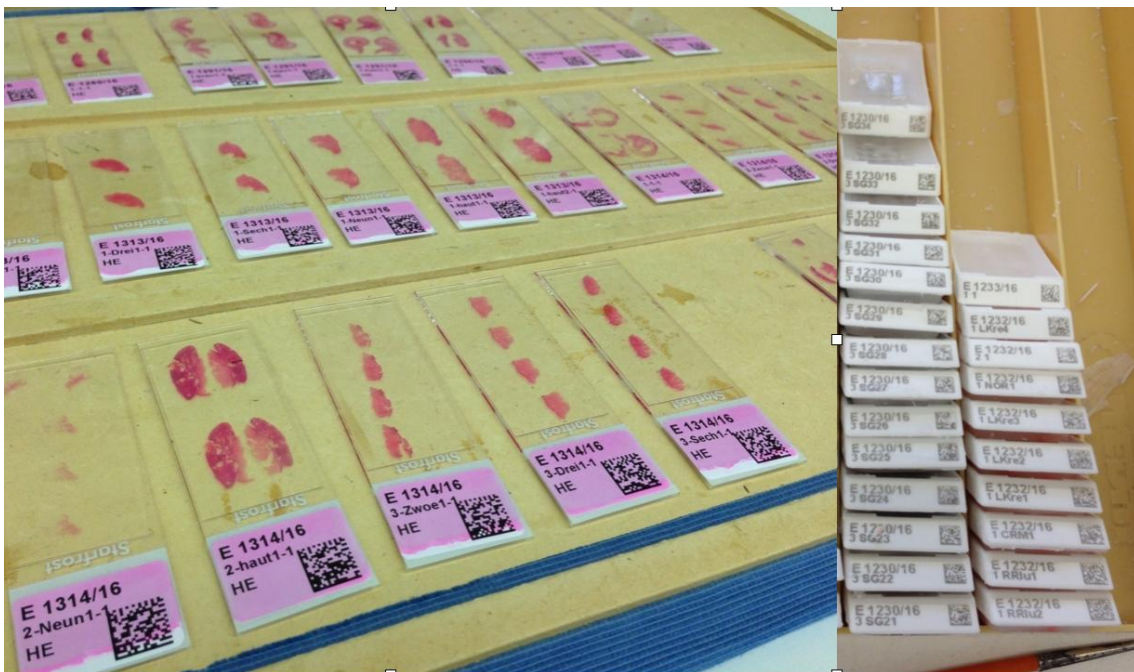
Figure 5: 2D-Barcodes on slides and cassettes in the laboratory routine. For human readability reasons there is also plain text printed on the labels and cassettes, demonstrating the quadruplets of IDs.
