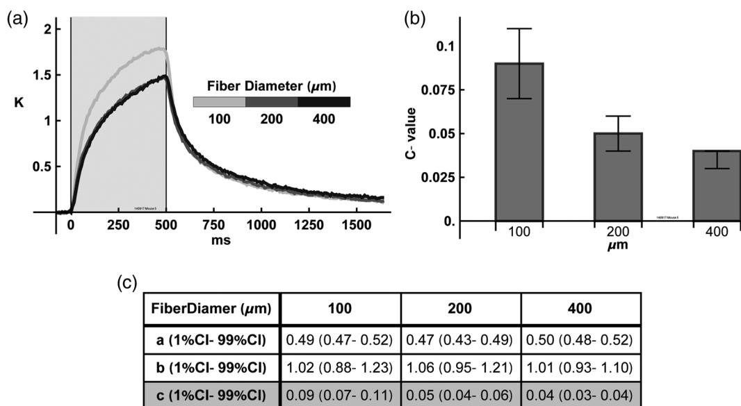
**Fig. 3** Effect of fiber diameter on heating. (a, b) Thinner fibers have higher local irradiance and therefore induce more local heating, in general. No clear difference is seen between 200 and 400  $\mu\text{m}$  fibers, likely due to the unavoidable illumination of blood vessels with larger fiber sizes (see text). Plots and error bars are as in Fig. 2. (c) Table representing the model fit values. Changes are mainly seen in the **c** parameter.
