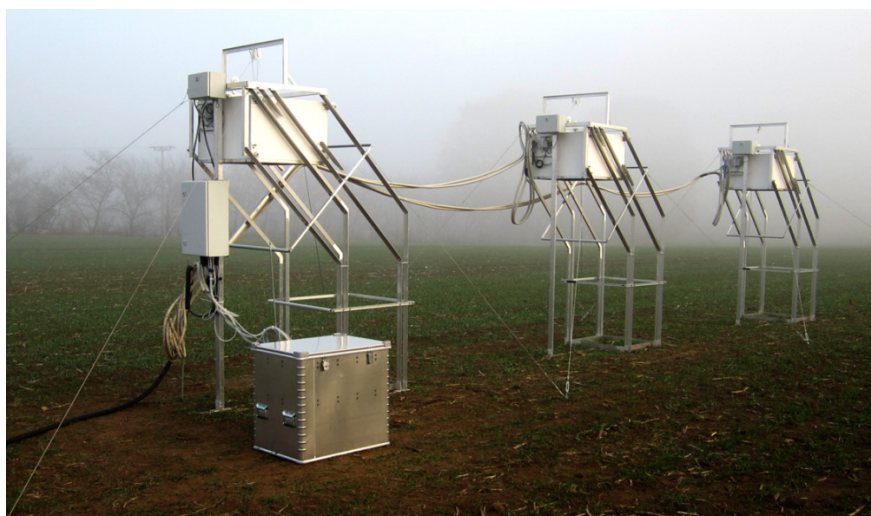
Figure 12: Greenhouse gas measurements using automated chambers
