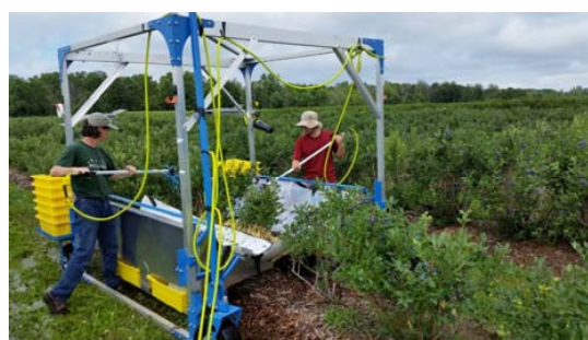
Figure 3. Harvesting blueberries with a semi-mechanical harvest-assist system consisting of hand-held pneumatic shakers to detach fruit and platforms to collect detached fruit. The frame is manually pulled/pushed over plants and the fruit catching platforms are pulled out while positioning the frame over the plants to be harvested and pushed towards each other to seal around the base of blueberry plants. Shown here are two workers harvesting blueberries with hand-held shakers. The yellow hoses carry pressurized air from a compressor to shakers. Yellow fruit lugs are positioned below the catching surface. The inclined catching surface diverted detached fruit into lugs.
