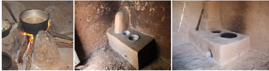
Figure 2. Examples of a TSF stove (left); an initial ICS (middle); and a modified ICS (right).
