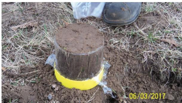
**Figure 4.** Undisturbed soil sample with 12 cm diameter.
