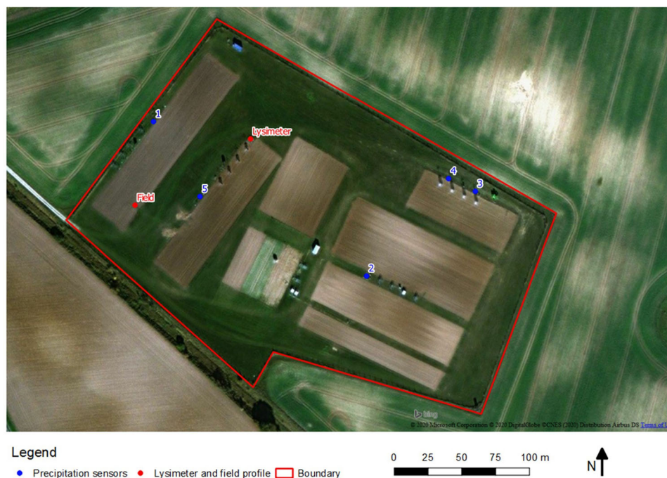
FIGURE 2 Aerial image (capture date range: 30 June 2010 to 19 Sept. 2016) and map of the experimental field site (CarboZalf-D) located in northeastern Germany; the locations of the rain gauges and the “field” soil profile and “lysimeter” station. Locations of rain gauges for measuring precipitation are numbered (1–5), and instrument types are described (Table A2)
