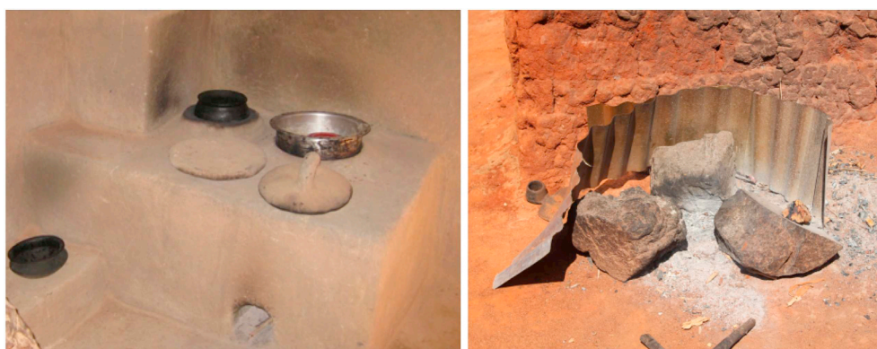
Fig. 1. Improved cooking stove (ICS) with a two-pot design and one fire chamber (left), three-stone fire stove with insulation sheet (right).
