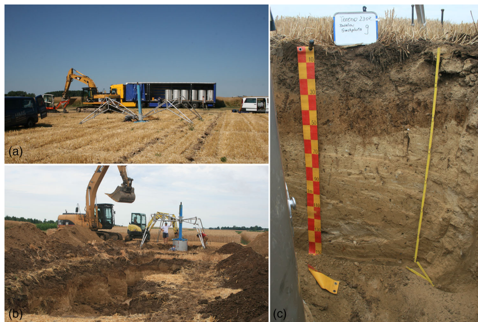
FIGURE 2 Photo of (a) the Dedelow site before, and (b) after lysimeter extraction July 2010. (c) Typical soil profile with Ap-, Bt-, and C-horizons of the Luvisol. In the back of Photos a and b, the instrument for lysimeter extraction can be seen. In Photo a, an air-suspended truck is shown, which was used to transport the excavated soil monoliths to the experimental research field station in Bad Lauchstädt and Selhausen. Photo by Wilfried Hierold, Leibniz Centre for Agricultural Landscape Research (ZALF), Müncheberg
