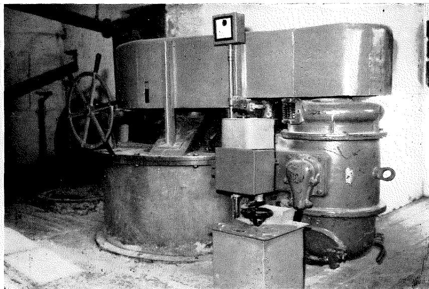
Figure 3. Machinery for production of binders from wood waste by a simple mechano-thermic process.
