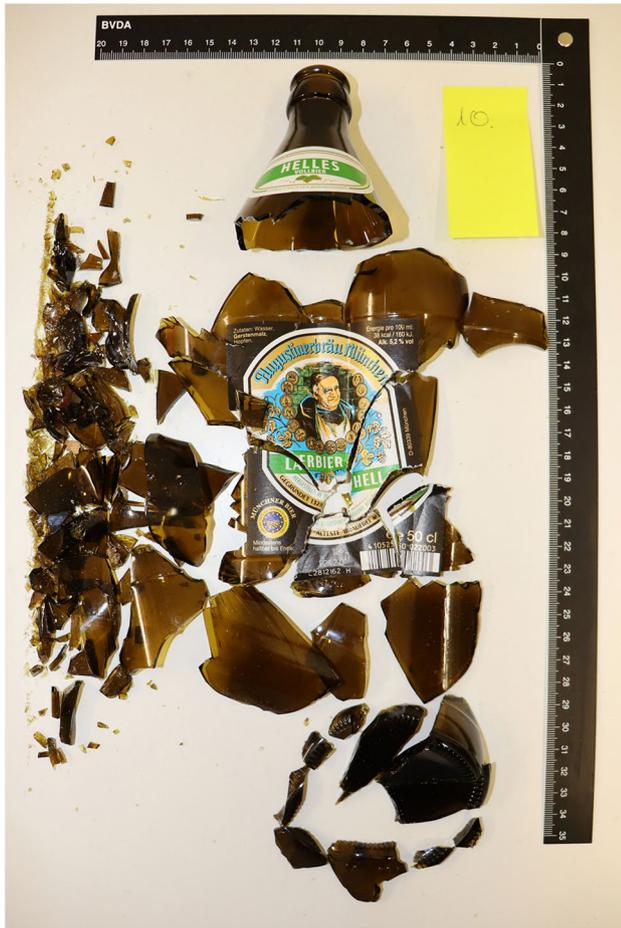
**Fig. 4** Glass fragments of a fractured 0.5-l beer bottle
