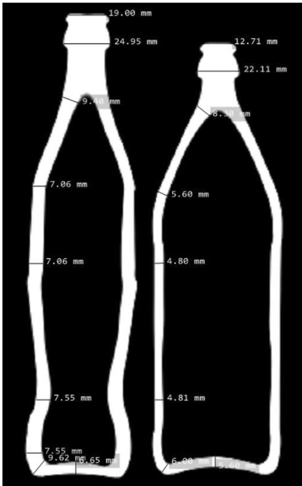
**Fig. 2** Axial slices of a CT scan of the used 0.5-l and 0.33-l glass bottles
