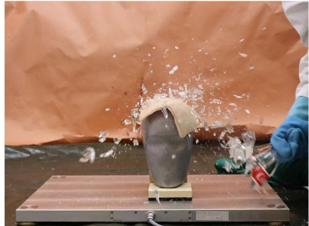
**Fig. 3** Fracturing 0.33-l Coke bottle when hitting the skull
