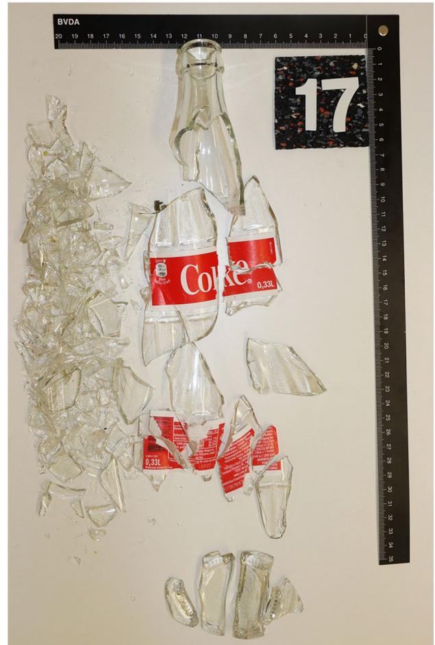
**Fig. 5** Glass fragments of a fractured 0.33-l Coke bottle
