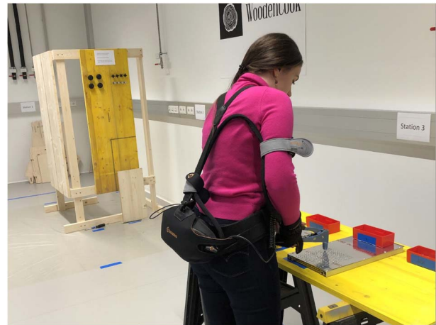
Figure 3. Exemplary picture of the experimenter executing one of the tasks while wearing the exoskeleton. Printed by permission.
