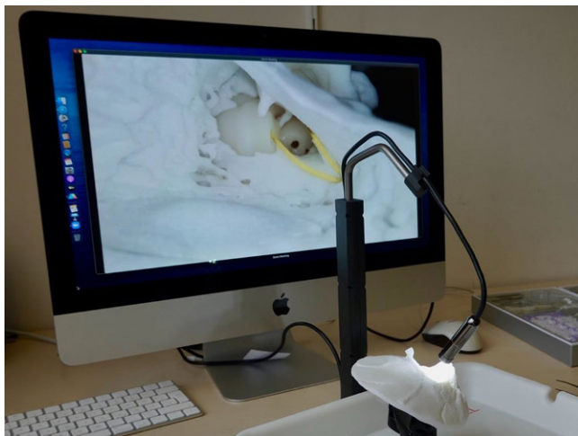
Fig. 1 ▲ The Online Temporal Bone Lab consists of an audio–video communication system, a macro camera, and an artificial temporal bone specimen
